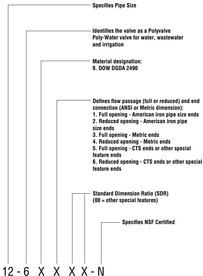
Special feature ends include integral socket ends, stub ends SDR, flanges, etc.
